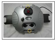
STEP 2: Unscrew the (2) Phillips screws from the topside of the cover.
