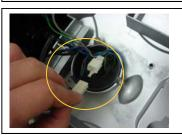
STEP 8: Disconnect the male/female plug that is connected to the UV-C lamp.
