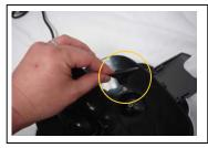
STEP 3: Pull off the Suction Cup from the underside of the Priming Lever.
