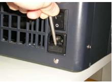
Insert (flat head) screwdriver and pull forward to remove fuse cover.
