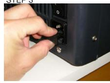
Pull out fuse cover that contains the spare fuse.
