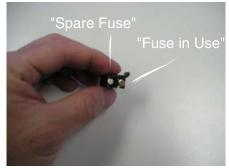
The "Spare Fuse" is shown on the left and the "Fuse in Use" is on the right.
