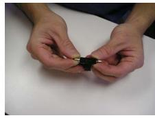
Insert the "Fuse in Use" into the side compartment to push out the "Spare Fuse".
