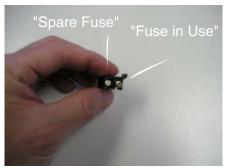
Insert the "spare fuse" into the "fuse in use" slot.
