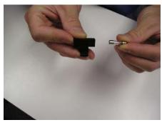
Remove "Spare Fuse" from side compartment.
