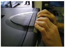
Put both hands on top of the controller and press down & forward to detach controller from chiller housing.
