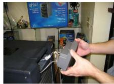
Reconnect with new replacement controller and connect Probe Sensor Wire & Power Supply Wire.
