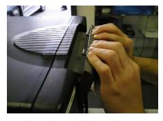
Insert controller back into chiller housing.
