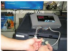
Dissconnect the Probe Sensor Wire.
